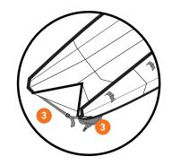
3 Pull off both fairings and fully loosen both end straps.
