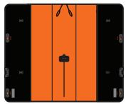
**6** Stern floorboard: Reinforces kayak bottom and holds the rear and middle seat.
