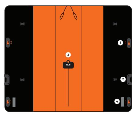
**Keyhole plates:** Hold the reinforcing rod in securely.
